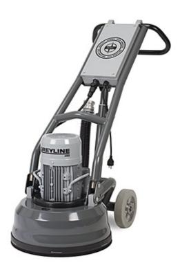
HTC Greyline<sup>™</sup> 450 is a single-phase, planetary grinder with three grinding heads and a counter-rotating grinding wheel for a stabile grinding without lateral forces. It works equally well for concrete grinding and floor prep as it does for grinding/sanding of wooden floors. The machine separates for easy transport.
